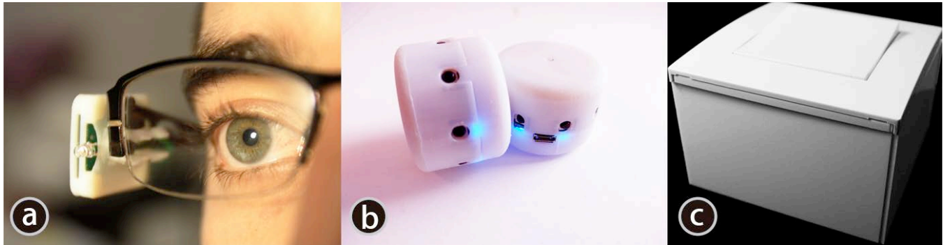
Figure 1: The InSight hardware components: a) the G-Ripple clip-on IR laser source; b) the G-Sens sensor to augment existing objects; c) example controller augmented with the hidden G-Sens sensor.
