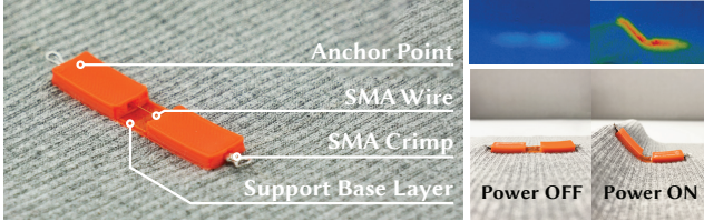
Figure 3: The composition of the ClothTiles's basic element. Anchor points assist keeping the rigidity of the element, meanwhile keeping the SMA wire in place with the support of the SMA crimps. When the current is applied, the generated heat (70°C) activates the SMA wire, thus the cloth actuates. The support base layer generates a bias force that brings the cloth back to its default shape when the power is off.
